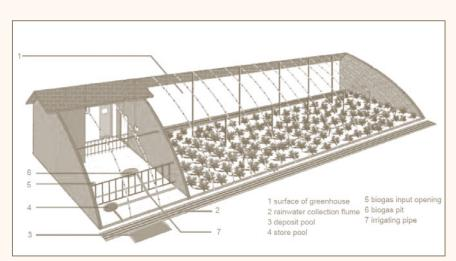
Structure of rainwater harvesting system (one greenhouse)
